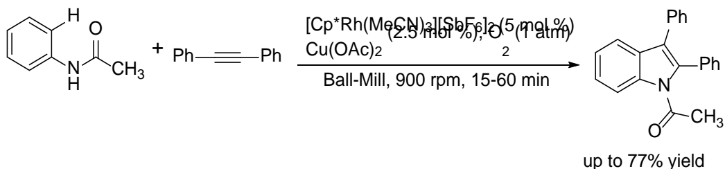
Scheme 19. Mechanochemical, Rh-catalyzed protocol for the efficient synthesis of indole derivatives
