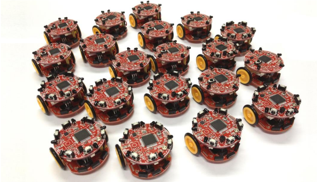
Fig. 15.3 Low-cost autonomous robots that mimic honeybee swarming behavior
